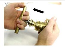
2.) Reattach handle to Stem and remove Stem Cartridge Assembly from valve Body. (If Stem is removed while Poppet and Seal Housing remain in valve Body, Poppet has been damaged during valve operation, consult factory).
