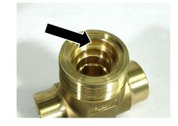
4.) Make sure body internal geometry is clean of dirt and debris. Lubricate face of valve Body that engages the 023-V75 O-ring and STBR-023 with Krytox GPL 205.
