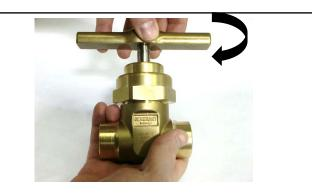
6.) Remove handle and replace bonnet. Tighten bonnet to 80 ft·lbs. Replace Handle and actuate valve to ensure smooth operation.
