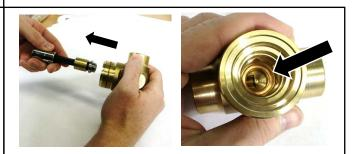
3a.) If seat replacement is necessary, use a 3/8" allen wrench to remove by turning clockwise (left hand thread). Inspect copper crush washer for damage and only replace if necessary. Carefully install new seat to 55 ft·lbs using care not to damage the seat.
